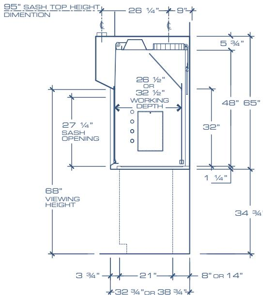
**Make-up air volume to the hood should be to a maximum of 70% of the exhaust volume**
