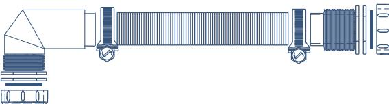
**FRONT POST MOUNTED PASS-THRU GROMMET**
