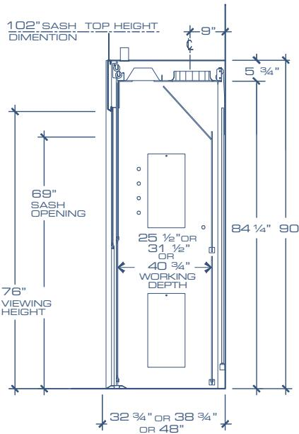
Exhaust air volumes are calculated with lower sash at closed position
