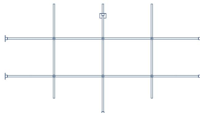
**Aluminum Distillation Rack assemblies for Bench Mounted Hoods**
