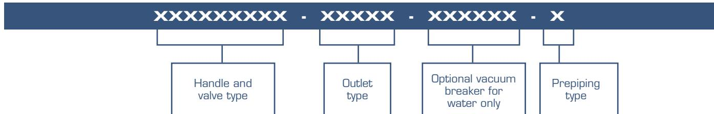
**PREPLUMP : Last digit of prelump kit # specifies the type of piping. Refer to the following chart for standard pre-piping.**
