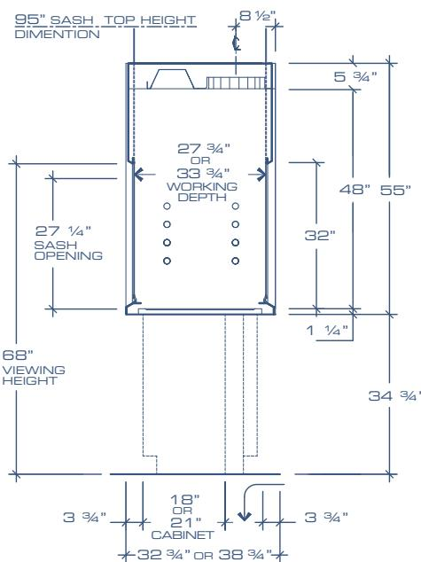
Exhaust air volumes are calculated using one side opening at the time
