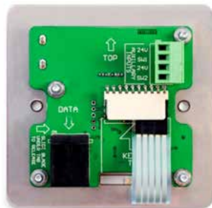
Figure 22 - Keypad/Alarm Panel Rear View
