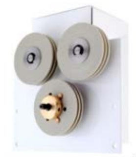
Figure 15 - Pulley and Wire Drive
